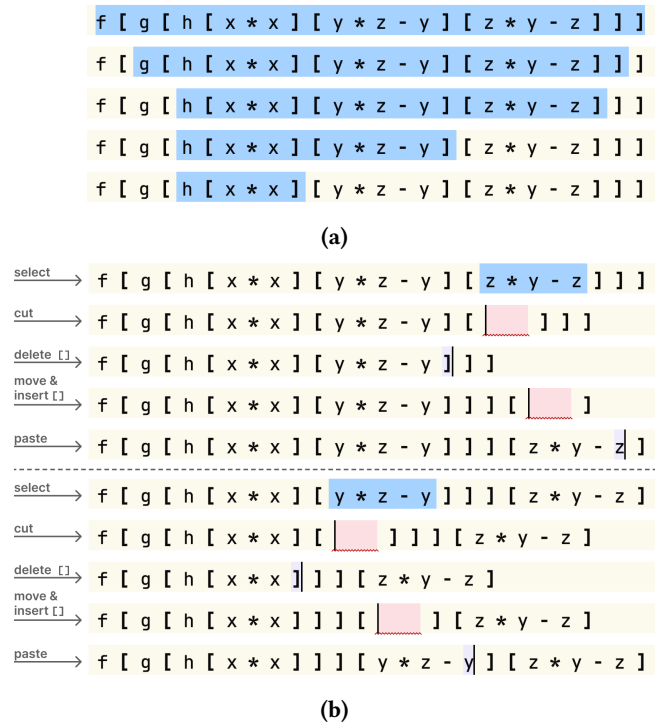
Figure 3. Screenshots of JetBrains MPS being used to edit a program expression of nested function applications, written in a small artificial language called Lamb that we used in our user study (Figure 7). (a) shows all possible selections the user can make that contains a bracket, given MPS’s restriction of selections to complete program terms. (b) shows the optimal edit sequence for completing one of our study tasks. The ultimate effect in the user-facing projection is swap the token ranges [ y * z - y ] [ z * y - z ] and ] , but selection restriction means the user must go through two separate procedures of cutting an argument, deleting its enclosing brackets, reconstructing the brackets elsewhere, and pasting.
